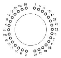
Bolt torque sequence (from above turntable)
