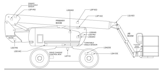
**LSA10S:** Limit switch, Axle #1 Oscillating Operational. Activates the axle oscillate circuit on the right side.
