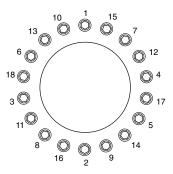
Bolt torque sequence (from below chassis)
