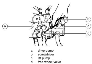
Note: The free-wheel valve should always remain closed.
